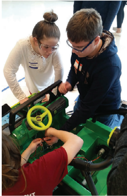
Students wire in a switch, electrical relay and a speed controller to modify this car for a child.
