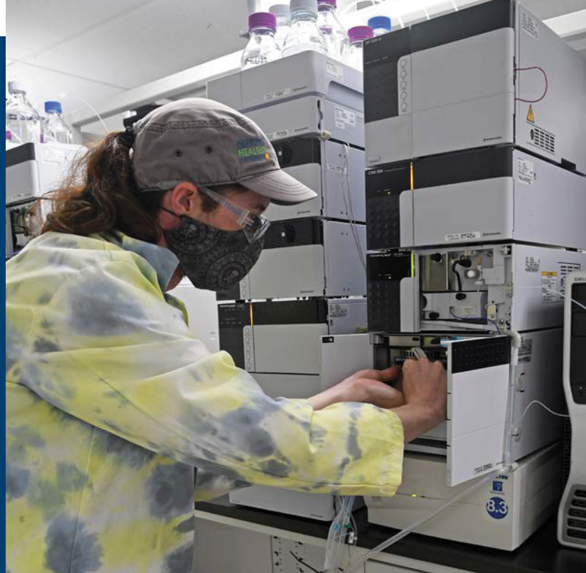
AMT R&D Technician Bob Moran installs a HALO® HPLC column.
